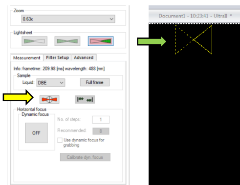
Figure 8.8. The horizontal focus can be moved to shift the location of the light sheet's waist (where it is narrowest in Z) in the X dimension.
